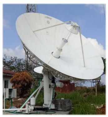
The antenna reflector is of dual shaped Gregorain configuration with corrugated conical feed horn and sub-reflector. The antenna meets the gain and side lobe specifications of International standards ITU-RS-580-6.
